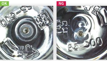
Picking out NG plastic bottle by inspecting the center position of its bottom
